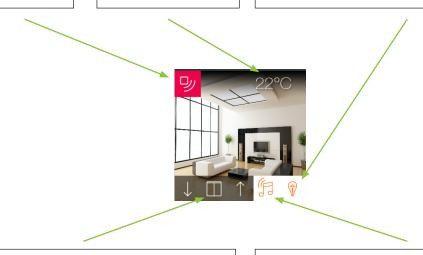
If a shutter or shutters are configured in the room, they are represented at the bottom left, the arrows enable the shutters to be opened and closed, a single click on the middle image causes a stop. The status, as for the site, is represented by all open, all closed or undefined position.
