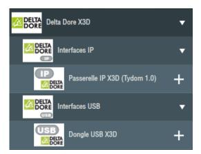
There are 2 X3D connectors available, a USB connector (USB key provided with the server) or an IP connector that corresponds to a Tydom I.O gateway. In both cases the configuration and functionalities will be identical.
