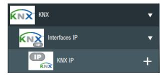
Add a new KNX/IP connector to the list using the corresponding "+" button.
