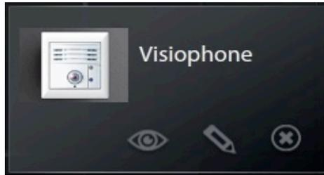
This device includes three buttons. The 'eye' button shows the video door station image following configuration. The 'pencil' button to edit the configuration of the videophone. The 'cross' button to delete the device.
