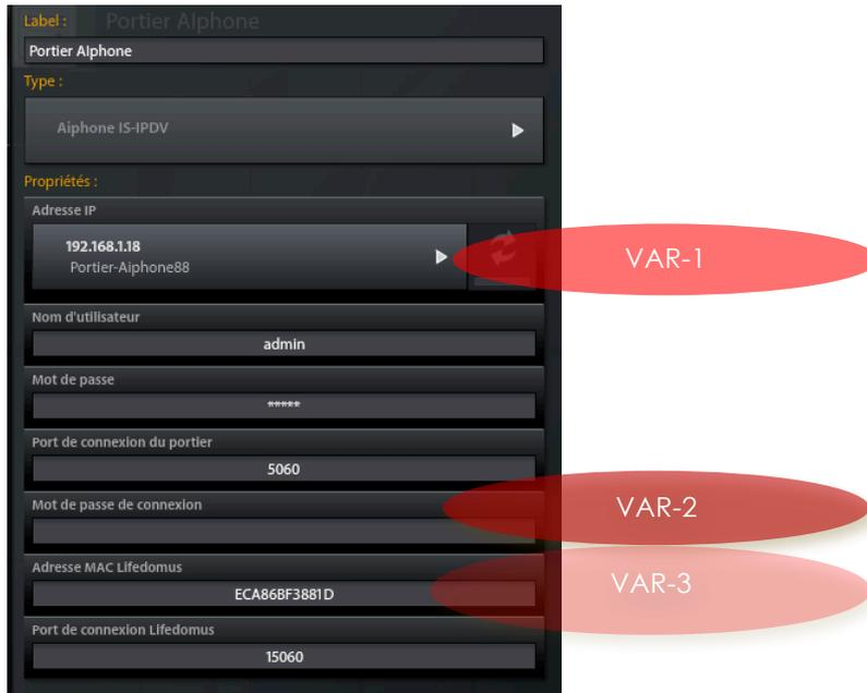
Fig. 4. Aiphone IS-IPDV videophone main configuration page
