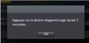
To start the association, press the teach button for 3 seconds. (The button is located at the back of your Somfy remote control).
