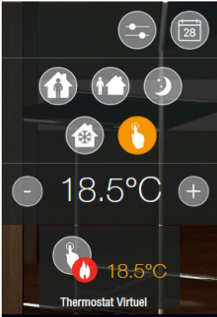
The temperature setting can be modified (by clicking on the + and - buttons), and one of the modes preset in the Config Studio can be selected.
